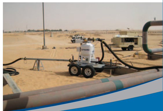
SX250-V Mobile Sludge Pump shown with rollcage (optional)
